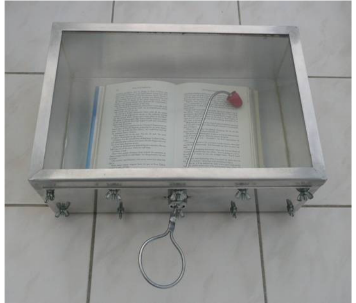
Reading Box A glass and aluminium reading box can enable someone sensitive to inks, chemicals in paper and/or fragrances left on the book by other readers to read a library book. The library book is sealed inside, held in place with masking tape along one edge of the plastic cover. Pages are turned with the rod. Photo: AESSRA
